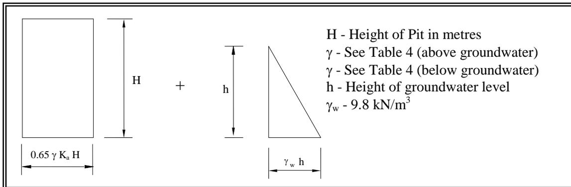
In calculating the lateral earth pressure for the shoring structure, the soil parameters are provided in Section 6.4.
