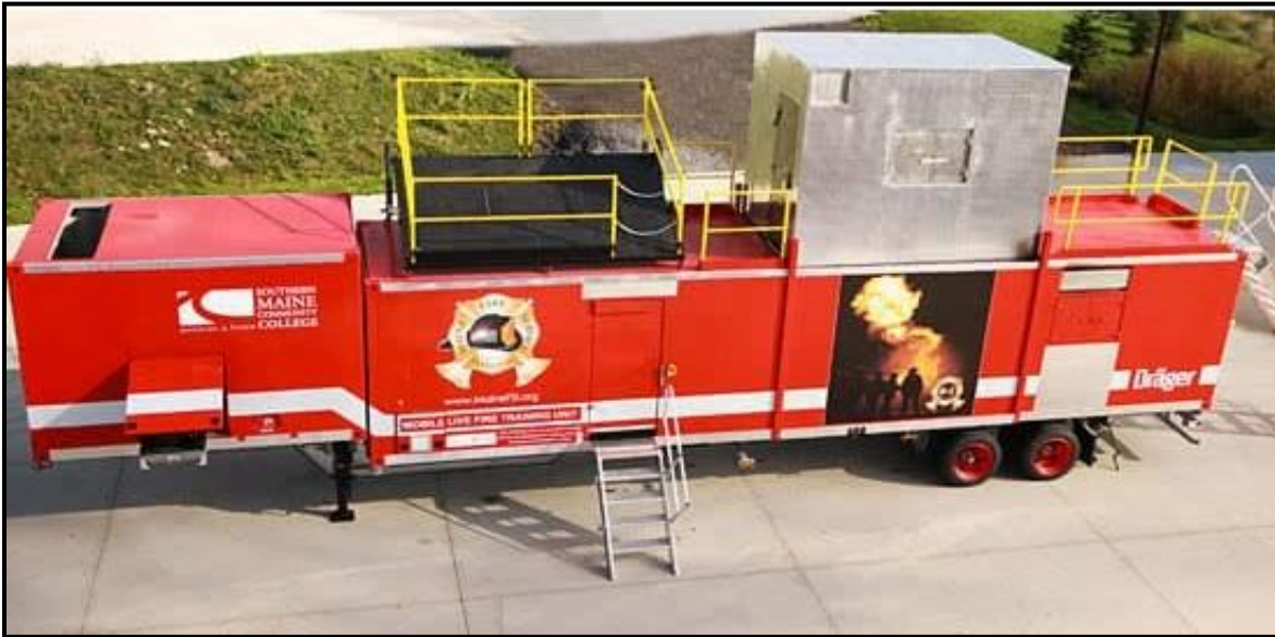
FIGURE 3: Example of Live Fire Training Unit – Propane Powered
