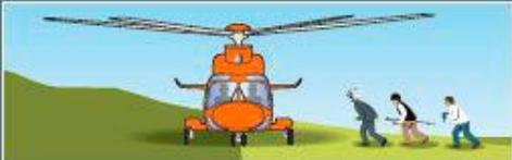
**IF ON UNEVEN GROUND**, approach or depart from the downhill side for maximum rotor clearance. **DO NOT RAISE ANYTHING ABOVE THE HEAD** and crouch while walking in the vicinity of the helicopter.
