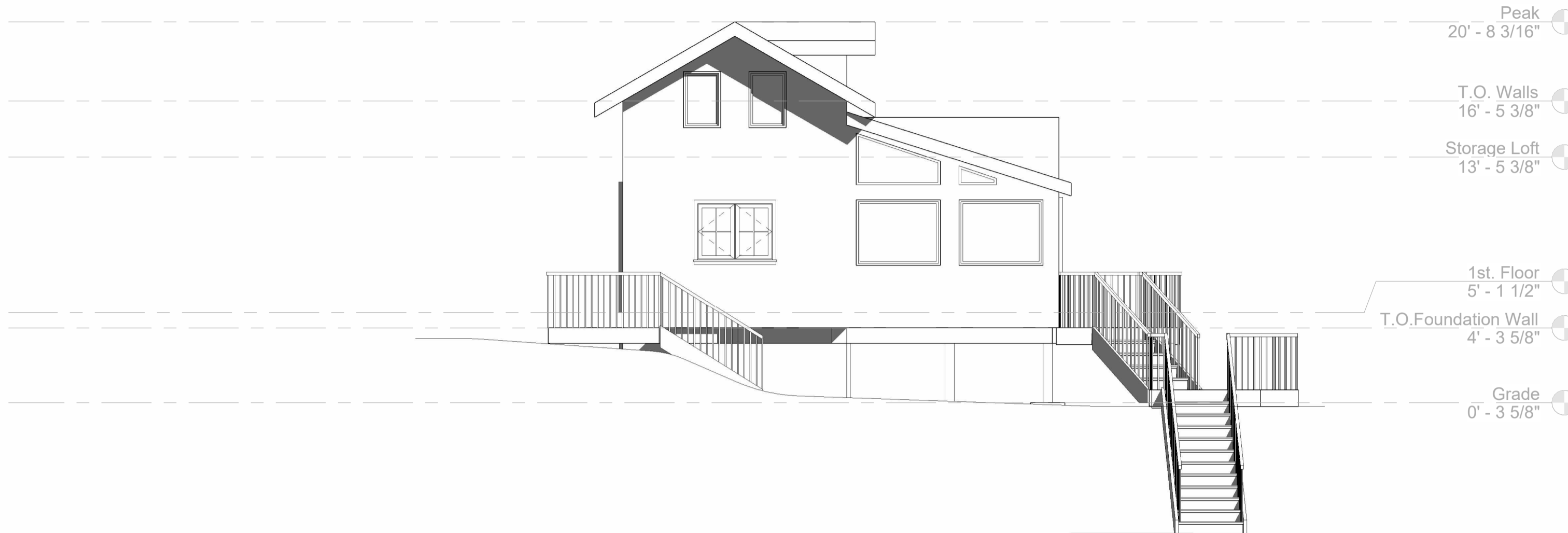
① Front Elevation 3/16" = 1'-0"
