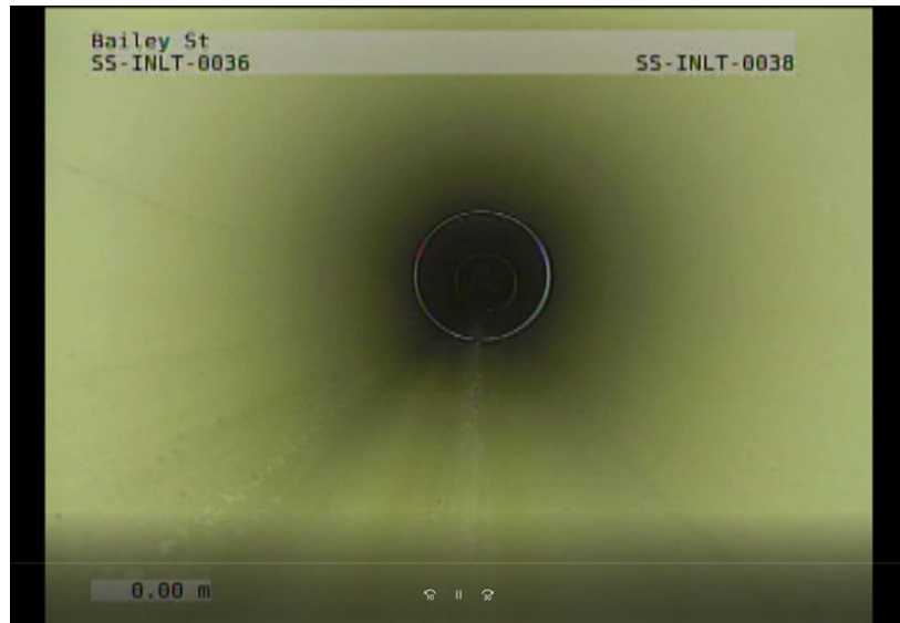
Figure 24: Good to Very Good No observed Defects (Condition Rating (CR) > 8.0)
