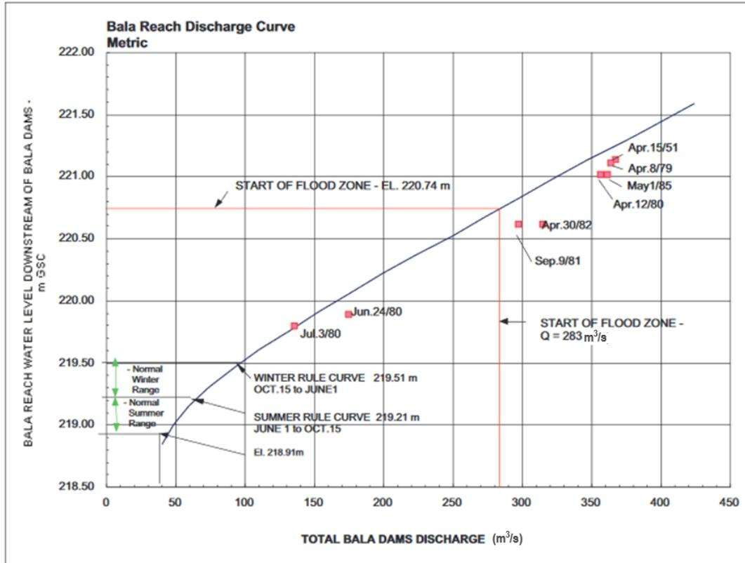
Figure 8. Elevation versus Inflow for Bala Reach<sup>25</sup>.
