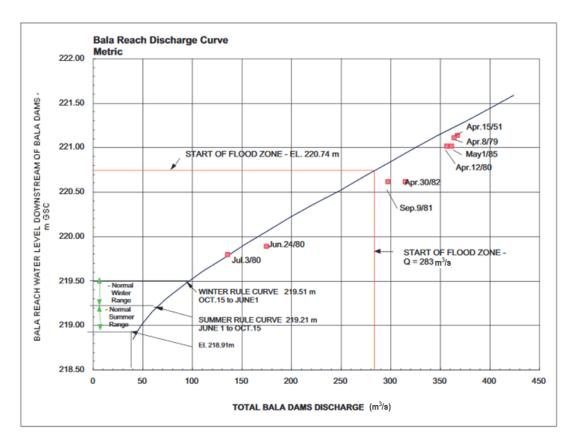
Figure 8. Elevation versus Inflow for Bala Reach<sup>25</sup>.
