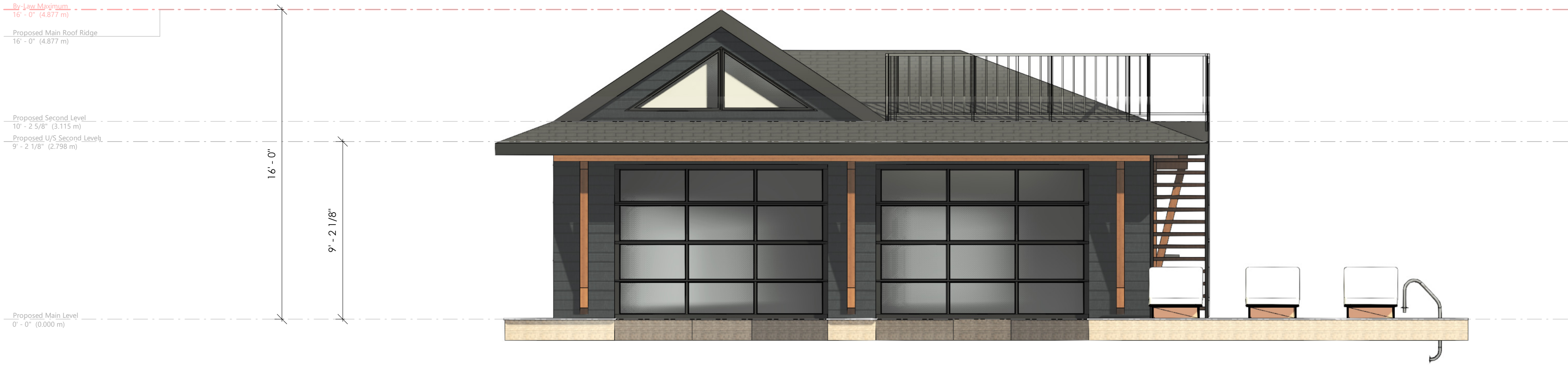
1 Architectural Front Elevation 1/4" = 1'-0"
